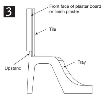
d) Position the tray in situation and level to the correct height as shown in diagram 4.
