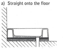
Important: This product must be bedded on a weak 5:1 sand/cement mix on a solid base of either concrete or marine ply in all installations. This smoothes out any undulations between the floor and the tray base.
