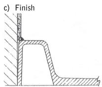
To prevent the possibility of water damage check all connections are watertight and that the tray is adequately sealed along the tiling line
